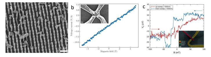
Fig. 1 (a) A representative SEM image of  $Pb_{1-x}Sn_xTe$  nanowires grown from a patterned mask. (b) A magnetoconductance graph of a  $Pb_{1-x}Sn_xTe$  nanoflake measured in the Van de Pauw configuration. The inset shows a SEM image of the measured flake. (c) The tunnel voltage measured between the ferromagnet and a metal contact as a function of the magnetic field. The inset shows a false-color SEM image of the measured device
