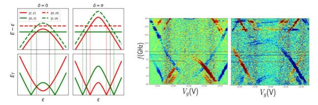
Fig. 1. Left: model of the junction and the ancillary level (top row: energies of the many-body states with even/odd parity in each subsystem; bottom row: corresponding allowed transitions). Right: Two-tone spectroscopy over gate.
