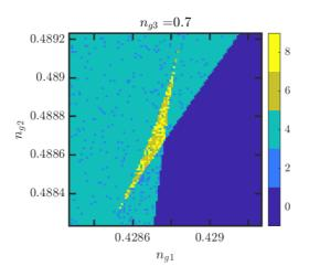
Figure 1. Number of Weyl points in the magnetic flux parameter space of a Weyl Josephson circuit with respect to offset charge perturbations. This shows the merging processes of 4 Weyl points nearby which draws a swallowtail singularity.
