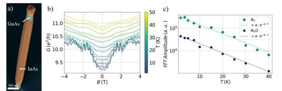
Figure 1 a) Electron micrograph of a GaAs/InAs core/shell nanowire. b) Magnetoconductance oscillations at various temperatures. c) Amplitude of Aharonov-Bohm oscillations vs. temperature and fit according to a quasi-ballistic transport regime.
