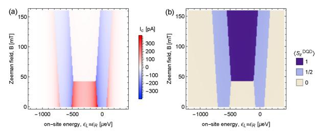
Figure 1. (a) Magnetic stability diagram of the double quantum dot Josephson junction; (b) Ground state expectation value of the z-component of the total double quantum dot spin reveals that the supercurrent is blockaded in the triplet configuration.
